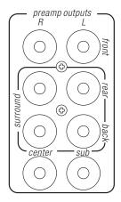
Surround Rear Left and Right, and Surround Back Left and Right Preamp Outputs to your external amplifiers. The Subwoofer preamp output allows for connection to a sub-bass speaker system with its own external or integrated power amplifier ("active" or "powered" subwoofers).
