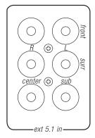
decoder's Center channel output to the Center channel input. Make sure to follow color coding of the plugs to ensure that both Center and Subwoofer are connected correctly; for instance, use the red plugs at either end to connect the center channel and the white plugs for the subwoofer channel.
